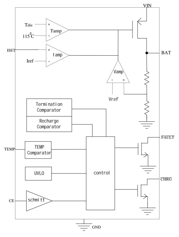
Figure 2 Block Diagram
