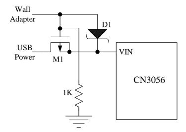
Figure 4 Combining Wall Adapter and USB Power
