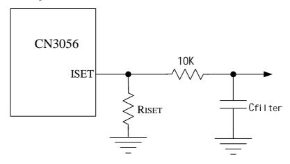
Figure 5 Isolating Capacitive Load on ISET Pin
